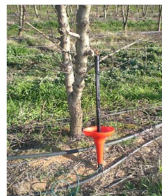
Fig 2. Monitoring root-zone nutrient and salinity using a wetting front detector (Fullstop).
